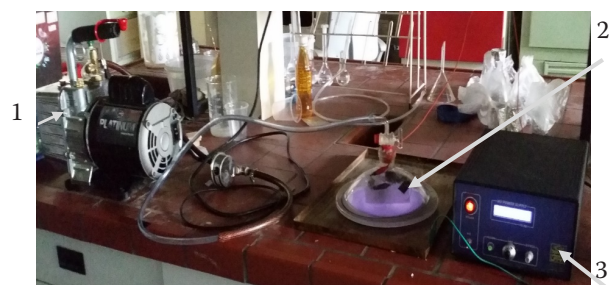
Figure 1. Vacuum plasma setup used in the experiment 1 – vacuum pump; 2 – plasma chamber; 3 – high voltage generator
