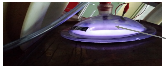
Figure 2. Seed placement location in the vacuum plasma chamber arrow shows embedded location for seeds
