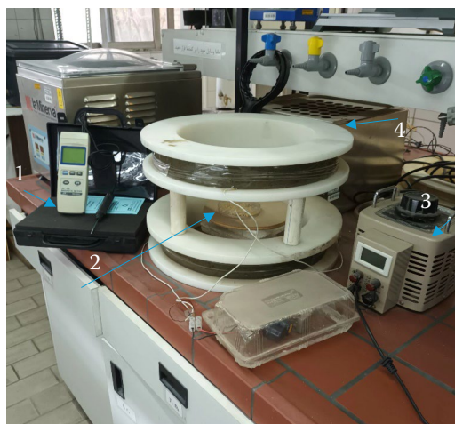
Figure 4. Electromagnetic setup used in the experiment 1 – Tesla meter; 2 – embedded location for seed; 3 – variac; 4 – Helmholtz coil
