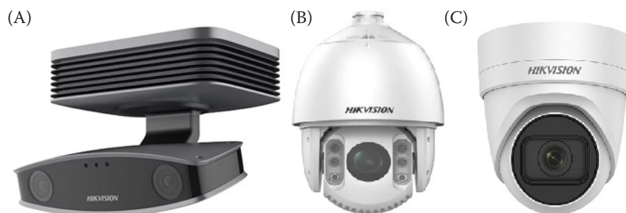
Figure 1. Tested recognition camera system: (A) HIKVISION iDS-2CD8426G0/F-I; (B) HIKVISION DS-2DE7232IW-AE(S5); (C) HIKVISION DS-2CD2H45FWD-IZS (2.8–12 mm)
