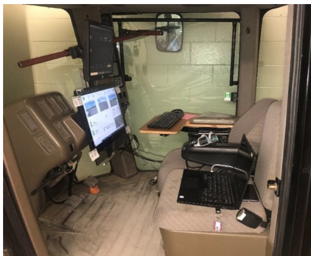
Figure 1. A tractor cab was used for the experimental study. Participants used the top monitor for the internet search task, while the bottom monitor displayed the simulation of the autonomous agricultural sprayer
