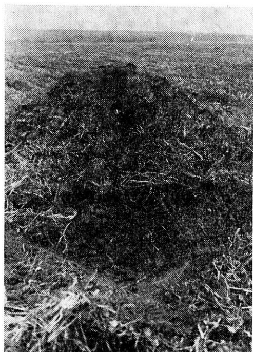
5. Nakyprenie pôdy s detailom v mieste vyhlbenia radlicou — Detail view of soil loosening at the spot of share penetration into soil
