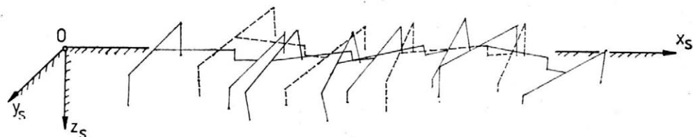
11. Priestorové polohy univerzálneho nosiča MT 8-046 pri jazde v smere vrstevnice, na svahu 17° — Spatial positions of the MT 8-046 general-purpose tool carrier when riding along the contour line on a 17° slope
