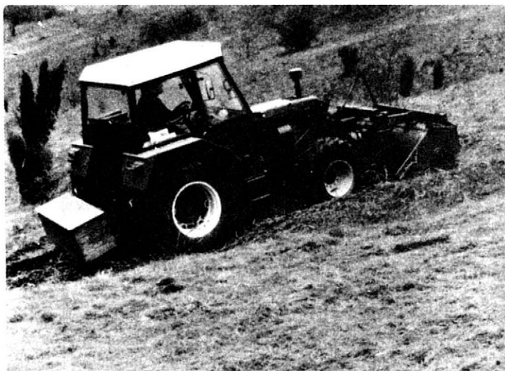
1. Ošetrovač povrchu PB 2-077 v agregácii s traktorom Z-7245 Horal pri práci na svahu 15° – Surface trimmer-crusher PB 2-077 in aggregation with the tractor Z-7245 Horal during the work on a 15° slope
