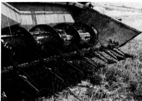
2. Paralelogramové zdvíhače JS-2 namontované na každom piatom prste žacieho stola – Parallelogram lifters JS-2 – mounted to each fifth finger of the cutting table
