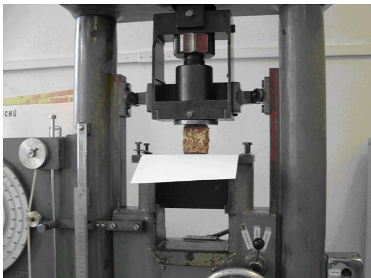
Figure 4. Briquettes mechanical properties testing by universal tearing machine ZDM-5
