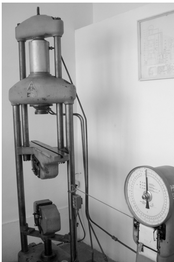
Fig 1. Compression device ZDM 50-2313/56/18 and pressing vessel with a plunger (Source: Department of Mechanical Engineering, Czech University of Life Sciences, Prague, Czech Republic)
