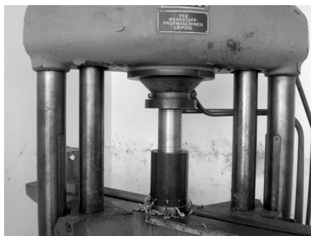
Fig 1. Compression device ZDM 50-2313/56/18 and pressing vessel with a plunger (Source: Department of Mechanical Engineering, Czech University of Life Sciences, Prague, Czech Republic)
