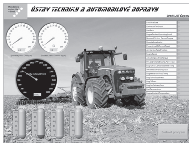
Fig. 3. Front panel of the software used for CAN listening
