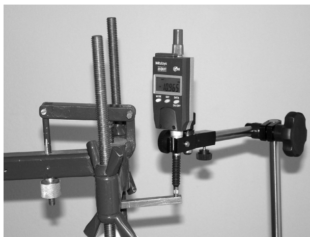
Fig. 1. Instrument for the measuring of eggshell deflection
