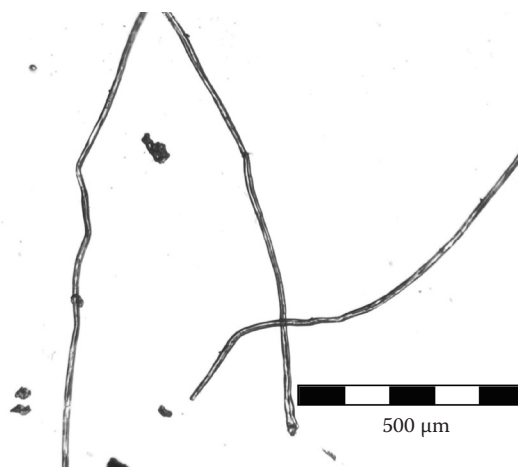
Fig. 1. Filler – polyamide fibre and rubber particles
