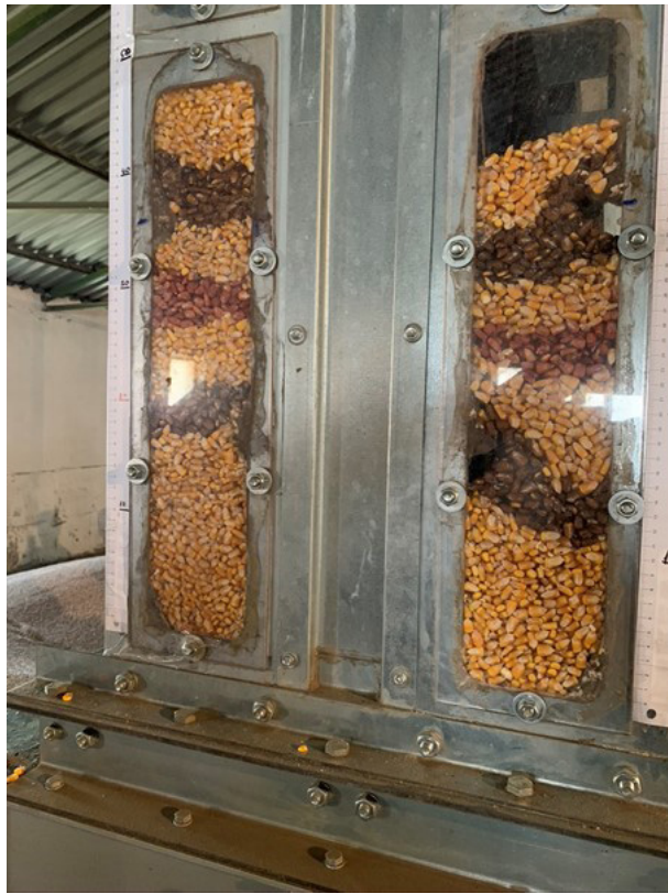
Figure 4. Distortion of the painted stripes due to the uneven particle flow
