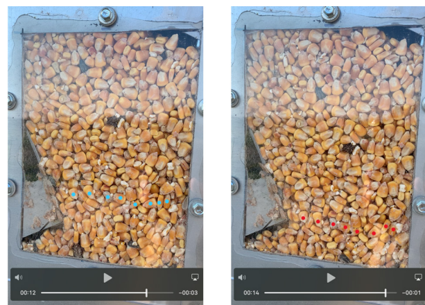
Figure 2. Vertical displacement value measurement method using video recordings
