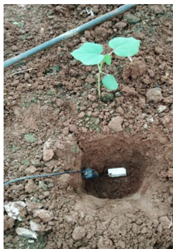
Figure 4. Sensor installed in the crop root zone
