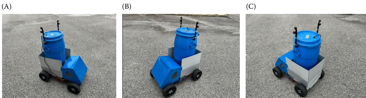
Figure 7. (A) Top view; (B) front view and (C) side view of the final version of the Auto Sprinkler Rover prototype
