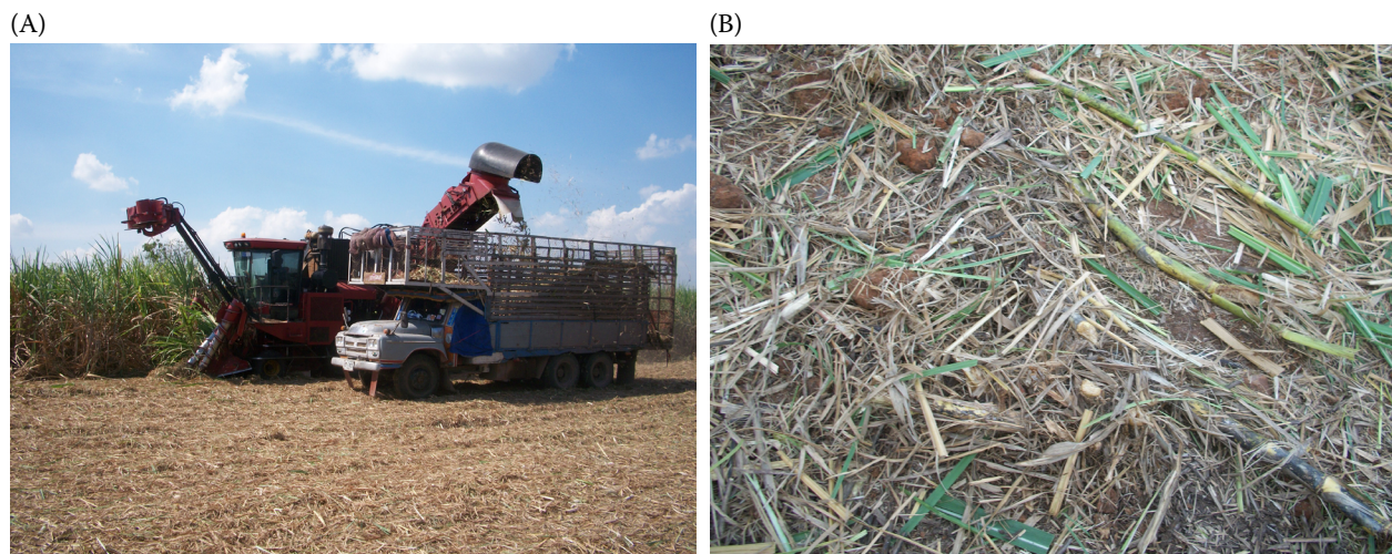
Figure 1. Mechanical harvesting operation: (A) chopper-type harvester performing green cane harvesting with simultaneous truck loading; (B) post-harvest field surface showing residual plant material distribution
