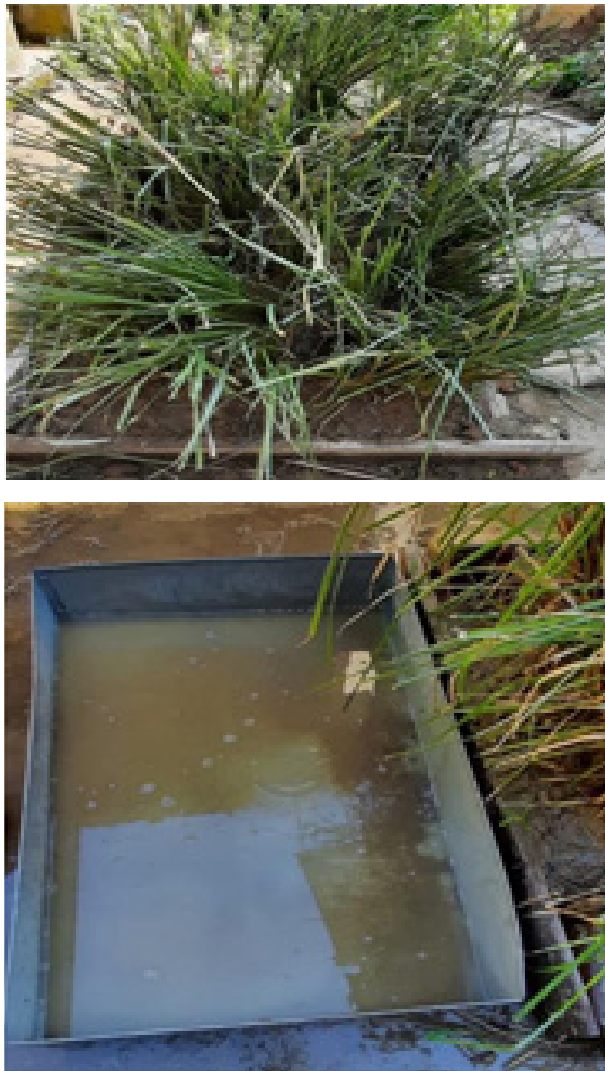
Figure 4. Vetiver grass plot on a micro model plot and the runoff accumulation after the simulated rainfall on the vetiver grass plot
