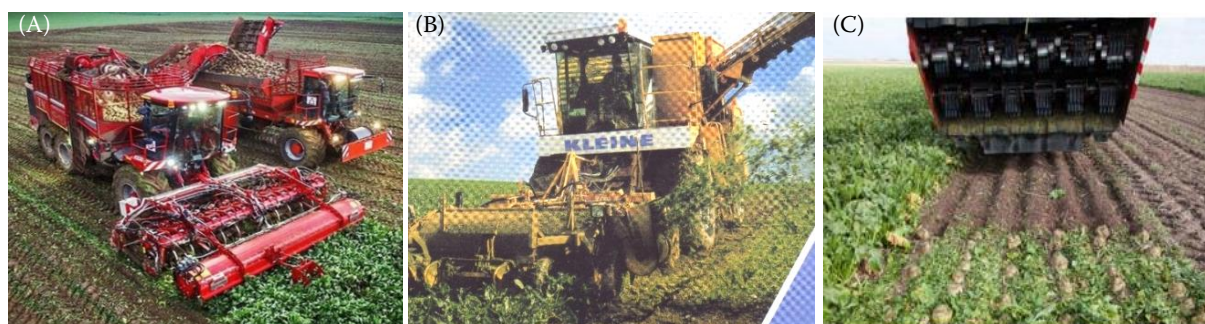
Figure 1. Existing methods of the primary haulm collection in root crop harvesting: (A) depositing the haulm into a windrow on the harvested field, (B) scattering the haulm over the harvested field, (C) placing the haulm into the inter-row space of unharvested root crops
