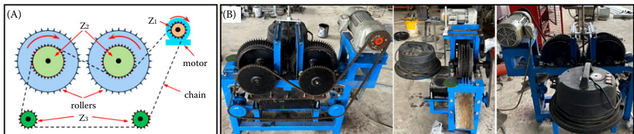
Figure 7. Chain drive system (A), fully assembled prototype machine (B)
