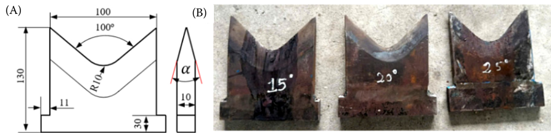
Figure 5. Geometric parameters of the cutting blade: specific cutting blade dimensions (A), three cutting blades used in the study (B)
